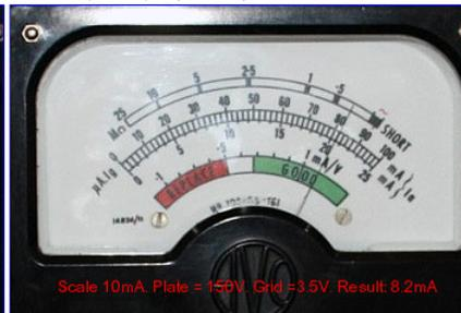
Scale 10mA, Plate = 150V, Grid =3.5V, Result: 8.2mA
