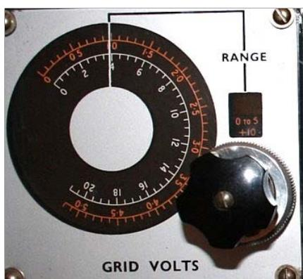
Now comes the grid voltage repair. With this setting, there is a small overlap with the settings wheel. So when the range is: 0 to 5 (+10) as picture here, you can set it from 10 to 15 Volt on the red scale. The next higher range is 0 to 5 (+15). so you can set it from 15 to 20 Volt.
