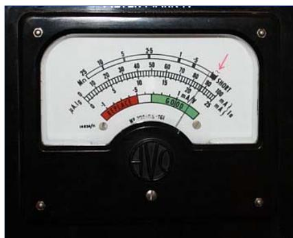
**It didn't work.** The calibration mark could not be reached with the SET~ switch now. I could only reach it I set it back to 190..210V. So what did this stinky seller do.... he just set the tester for 190..210, and that way, with 230V he could force the needle to the Calibration mark. Thus "fixing" the problem with the non-working mains calibration.
