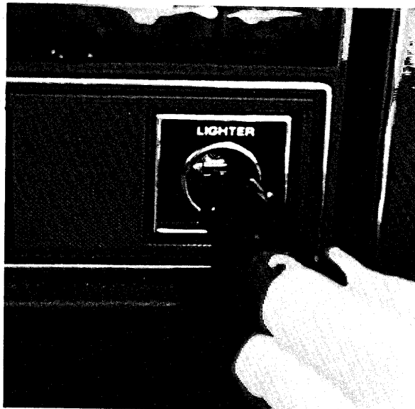
Fig. 7: The FC71 may be powered from an automotive accessory jack by using the supplied DC Power Supply Leads.
