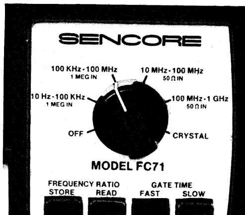
Fig. 15: Frequencies between 10Hz and 100MHz are measured using the 1 megohm input.
