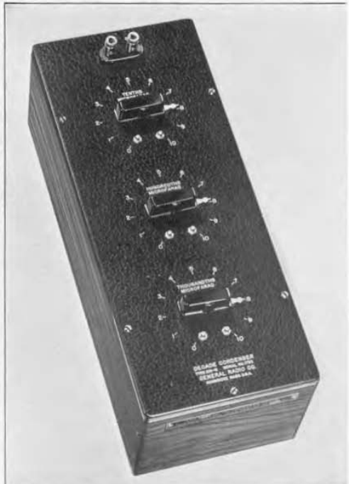
FIGURE 1. Panel view of a TYPE 219-M Decade Condenser.
