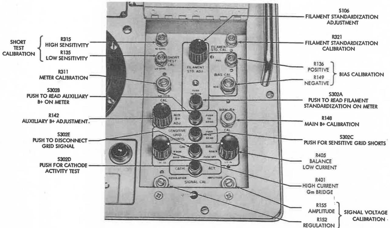
Figure 3 - Auxiliary Compartment
