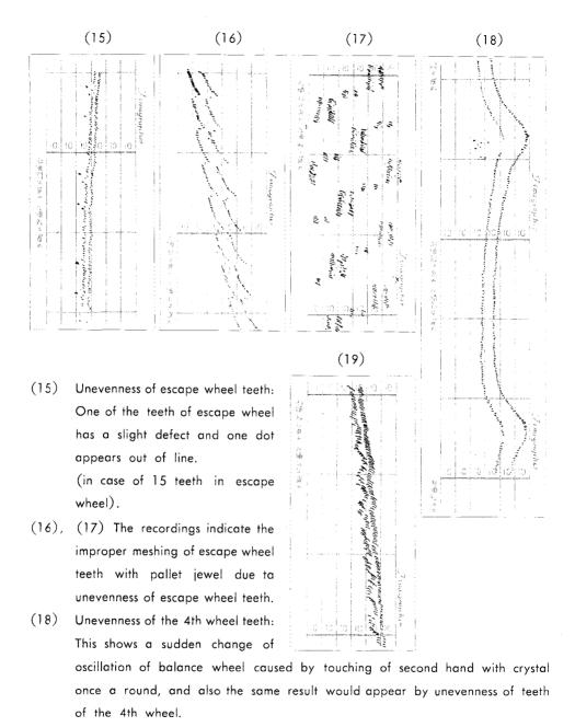
(19) Condition of banking pine: This watch loses 10 sec. per 24 hours due to some defects in esscapement. Impulse pin is not touching at fixed period with pallet fork due to maladjust-ment of banking pin and escapements.
