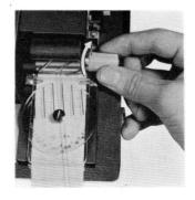
Gradually turn the volume control knob (H) clockwise, and the ticks will be heard, and a series of dots will appear on the recording paper.
