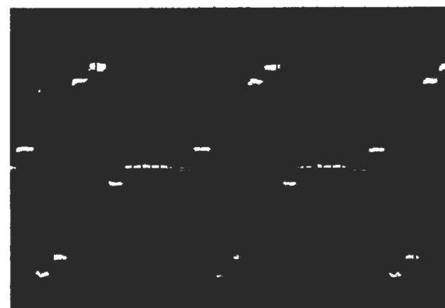
Fig. 29. Correct (R-Y) signal (red-colour difference signal)
