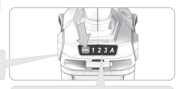
The "A" function is designed to give the user greater control in application and reduce damage to the fastener or work surface by automatically shutting the tool off after the tool senses the mechanism impacting for approximately one second.
