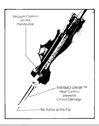
The Model PC-10 Desoldering System provides completely spike-free operation for the safe removal of components from printed circuit boards. Ideal for use with MOS-type devices, the system provides instantaneous, spike-free vacuum generation via simple finger actuation on the handpiece.
