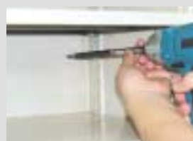
Tightening screws in high places or when nearby obstructions make work difficult.
