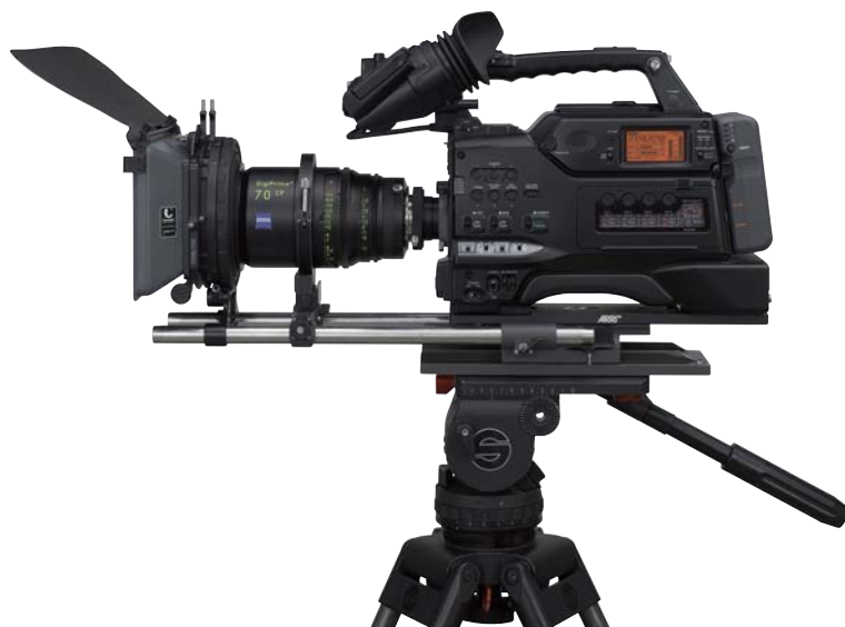
Cinema lens on HVR-S270P with an adaptor
