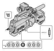
Lift up the bottom of the jack cover, then rotate in the direction of the arrow.
