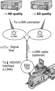
\* An i.LINK jack which is compatible with HDV1080i specification is required.
