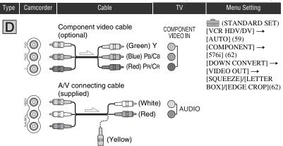
A/V connecting cable is also needed to output audio signals. Connect the white and red plugs of the A/V connecting cable to the audio input jack of your TV.
