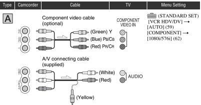
An A/V connecting cable is also needed to output audio signals. Connect the white and red plugs of the A/V connecting cable to the audio input jack of your TV.
