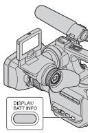
After a while, the approximate recordable time and battery information appear for about 7 seconds. You can view the battery information for up to 20 seconds by pressing DISPLAY/BATT INFO again while the information is displayed. Remaining battery (approx.)
