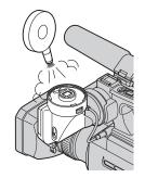
**3** Follow the reverse procedure of step 1. Align the I markings on the left side and attach the viewfinder by pressing it downward lightly. Then turn it clockwise until it is clicked.
