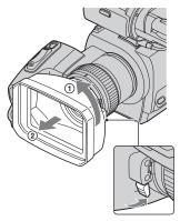
Turn the lens hood cover in the direction of the arrow as illustrated above while pressing the lever on the lens hood cover.
