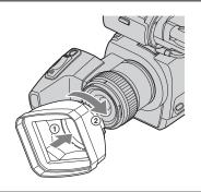
Align the marks on the lens hood to those on the camcorder, and turn the lens hood in the direction of the arrow.
