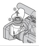
2 Remove dust from inside the viewfinder and the part shown below with a blower.
