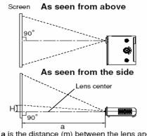
a is the distance (m) between the lens and the screen, and corresponds to a range of 1.20 m to 10.00 m. H is the height from the image bottom to the center of the lens.
