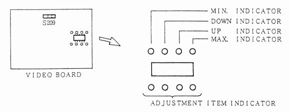
\* WHEN INDICATE THE BOTH LED OF MAX. AND MIN., IT MEANS CENTER.
