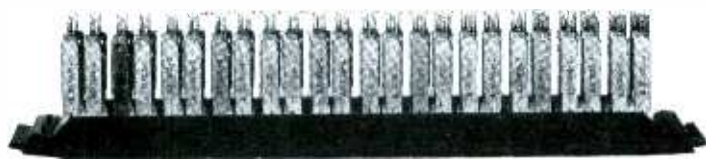
A Rear View of the 33-A Jack Panel
