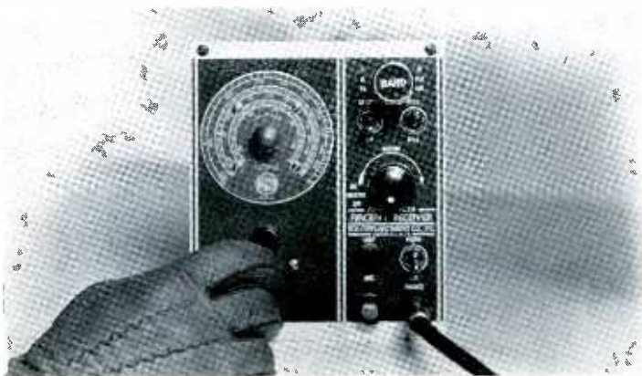
Remote control panel of AVR-7H. Panel can be split so that mechanical and electrical controls can be mounted separately.
