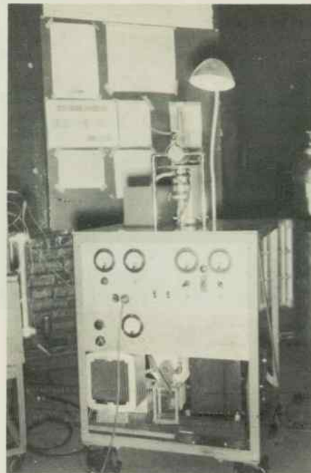
Scanning Microscope Equipped for Easy Change of Specimen
