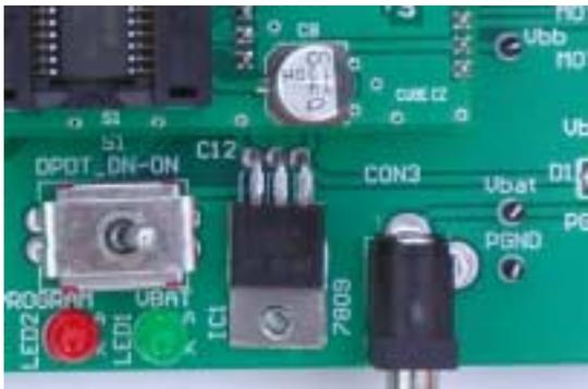
FIGURE 2.4 Toggling the Power-selection switch connects the DUT to the correct programming voltage. A red and green LED indicates the selected voltage.
