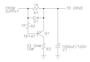
This circuit protects stepmotor and servomotor drives from damage during periods of energy return when operating near maximum rated voltage.
