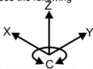
The "Y" axis is usually a "back and forth" movement, The "X" is usually "left and right" movement and the "C" axis is usually a rotary axis around the "Z" axis but it can also be used as a fourth axis in a foam wing cutter.
