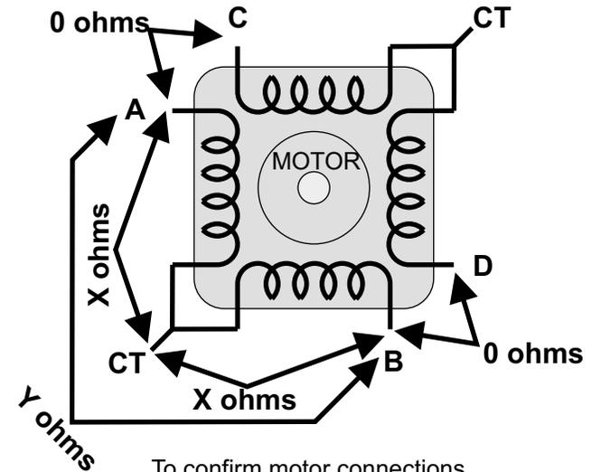
To confirm motor connections use a multi-meter and measure the resistance of the coils.
