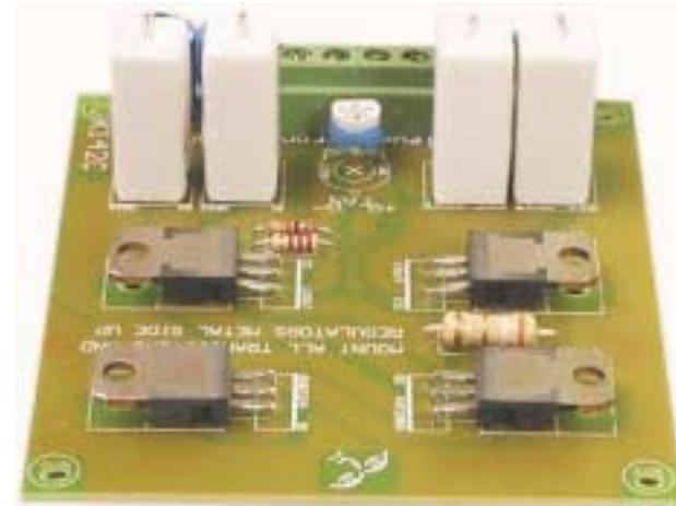
To change the current adjustment range select a new resistance for R6 and R7 using the calculation bellow. Remember that this will set the minimum current, you should select a minimum current below what is required so to allow for adjustment above and below the required current.
