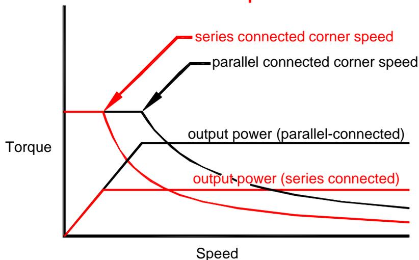
This shows a half winding connected motor delivers twice as much power as a full winding connection at a given power supply voltage. This is because full-winding inductance is four times higher than the half-winding inductance.
