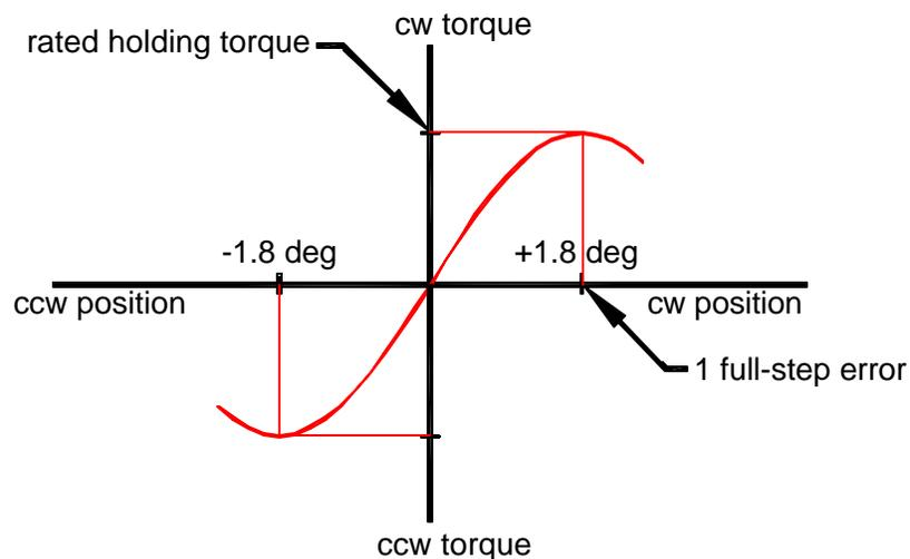
From this one may approximate that a static torque load equal to 15 percent of the holding torque will displace the motor shaft 1/10 of a full step about the origin.
