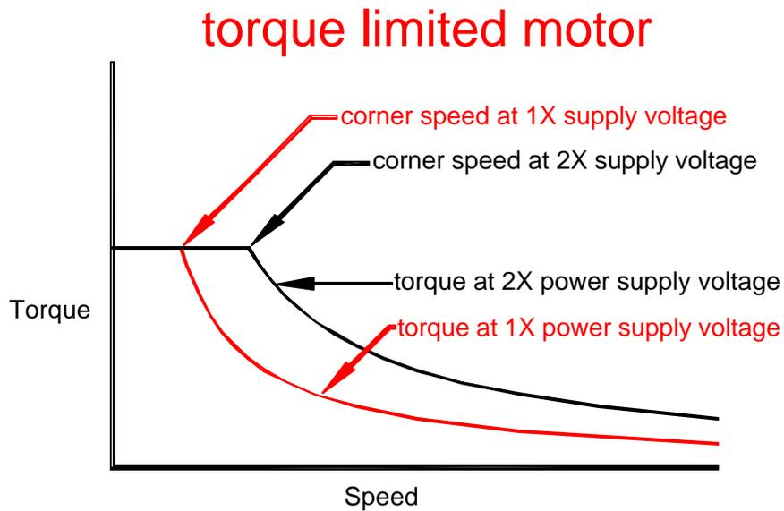
The result now is a two-part speed-torque curve which features constant torque from zero speed until it intersects the motor's natural load line, called the corner speed, beyond which the motor is in the constant power region.
