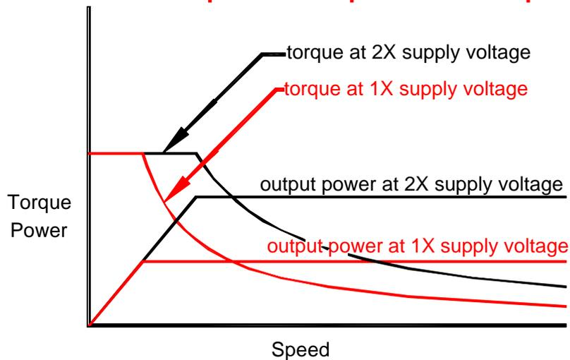
The following graph shows the effect of rewiring the motor from full-winding to half-winding while keeping the same power supply voltage.
