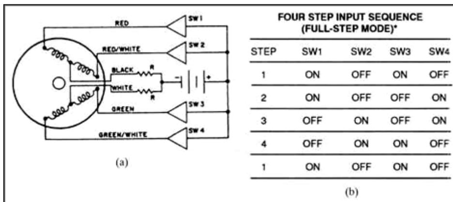
FIGURE 11-59 (a) Diagram of switching circuits for stepper motor. (b) The switching sequence for a four-step (full-step) switching mode. (Courtesy of Superior Electric, Warner Electric.)
