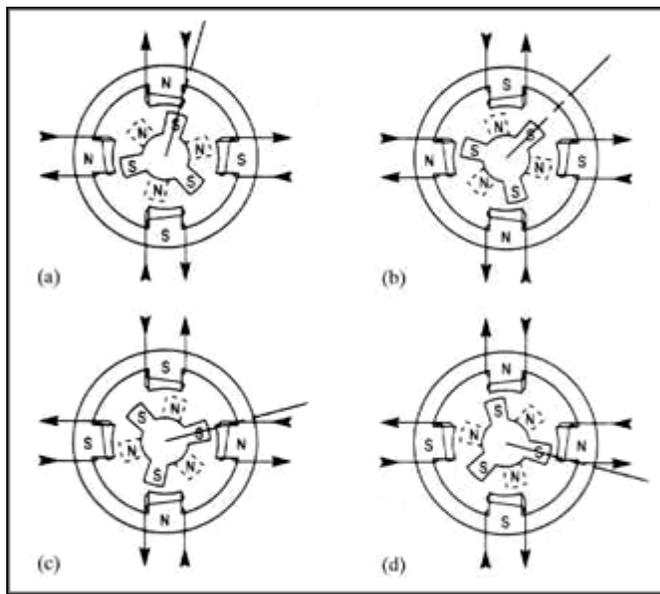
**FIGURE 11-60** The diagrams that show the position of each pole while the motor is in full-step mode. The diagrams a, b, c, and d show the movement of the rotor in sequence. (Courtesy of Parker Compumotor Division.)
