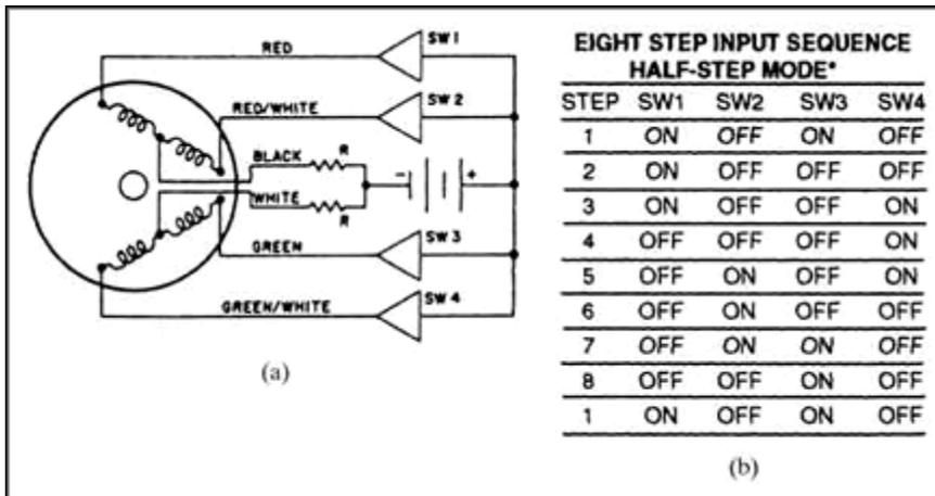
**FIGURE 11-61** (a) The stepper motor with its switches, (b) The switching sequence for the eight-step input (half-step mode). (Courtesy of Superior Electric, Warner Electric.)
