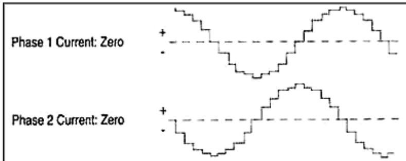
FIGURE 11-62 Phase-current diagram for a stepper motor controller in microstep mode. (Courtesy of Parker Compumotor Division.)
