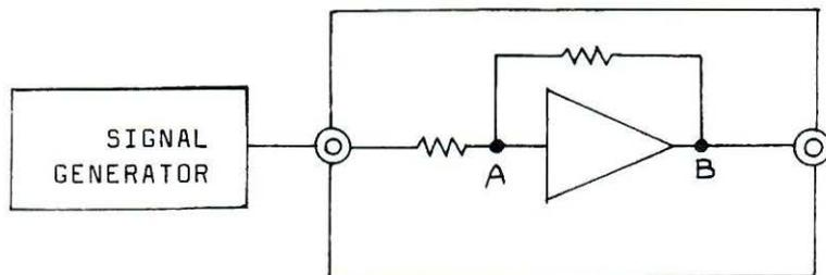
Figure 7 - Negative Feedback Amplifier Gain Measurement
