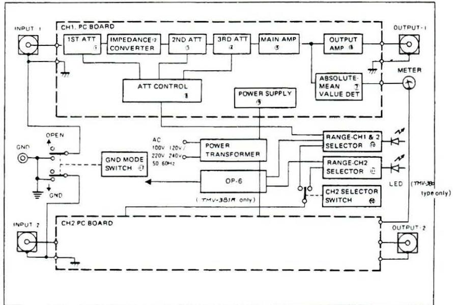
Figure 1 - Block Diagram
