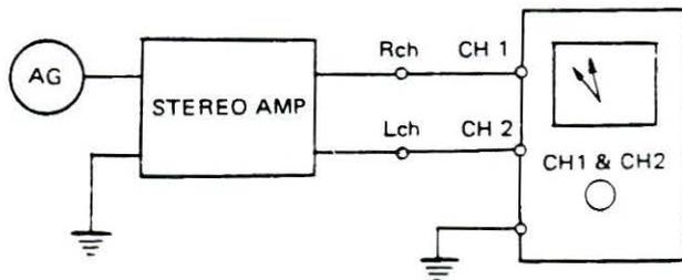
Figure 8 - Stereo Amplifier Frequency Response Measurement
