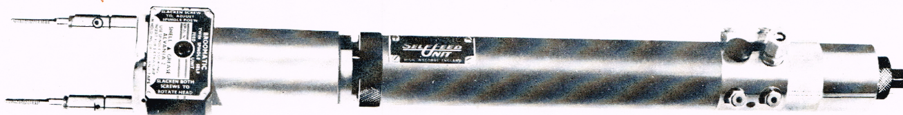
Twin spindle tapping head on Self-Feed Unit taper set for 2 1/2 in (63,5 mm) centres.
