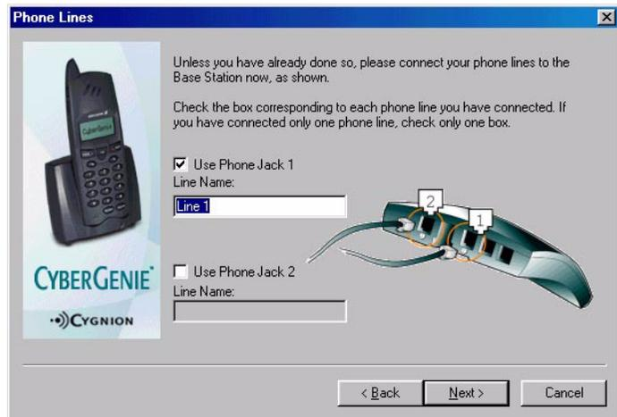
Make sure that the external phone line(s) are connected to the base station.
