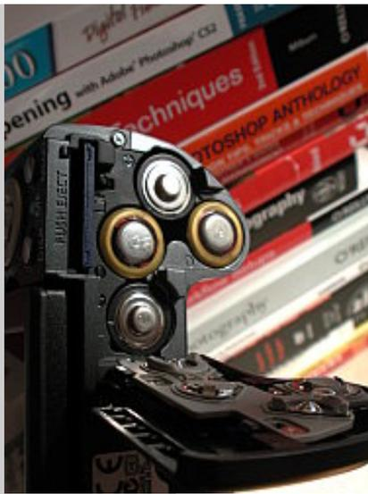
**Battery/Card Compartment.** The hinge is right next to the plastic tripod mount, but it's very easy to access either the card or batteries.
