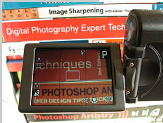
**LCD.** I'm holding the camera well below eye level to focus on the book spines, but I can easily see them because the LCD swivels.
