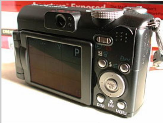
**Back.** The control layout is simple (not too many buttons) and easily managed with just your thumb. Luke was particularly happy to see that the Mode switch toggles between Playback and Record only, with Video moved to the Mode dial. After the shot, I flipped the LCD around so it looks like any other digicam.
