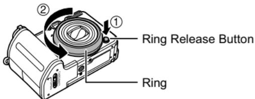
**3 When the ○ mark on the camera and the ◻ mark on the ring are aligned, lift off the ring.**
