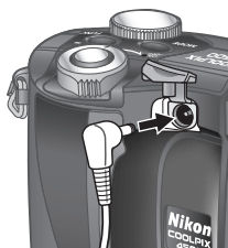
Connecting AC adapter to COOLPIX4500 DC-in connector
