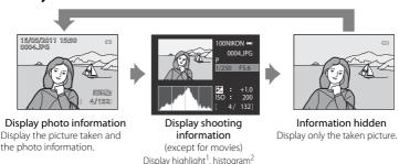
1 The brightest portions of the image (portions that are highlighted) blink. Use highlights as a guide when setting exposure.
