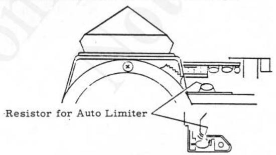
Protection against leakage current from M circuit board.
