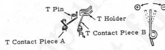
Adjust by bending T contact piece B
