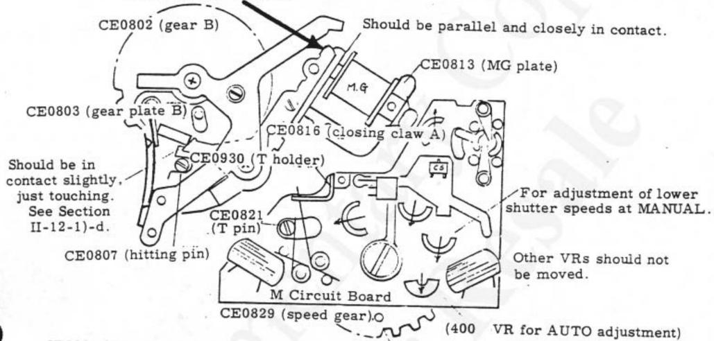
CE0821 (T pin) and CE0930 (T holder) are for the adjustment of higher shutter speeds at MANUAL.
