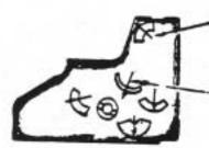
Comparator Adjusting VR (After setting to B, turn it from the film side.)
