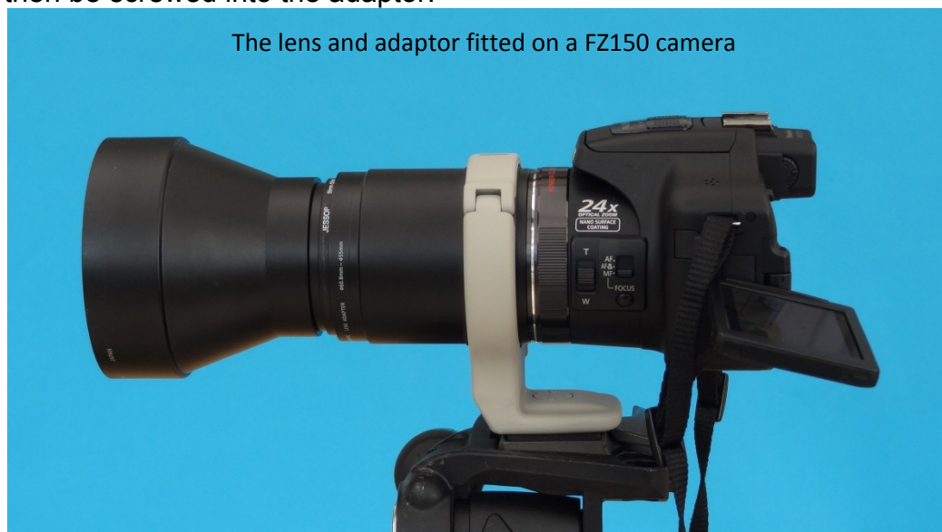
The Telephoto adaptor LTE-55 needs to be used with a DMW-LA7 Adaptor tube
