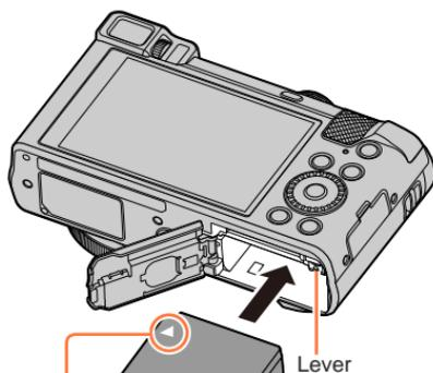
Make sure to insert the battery in the correct orientation.
