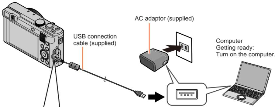
**When charging the camera, connect the USB connection cable (supplied) to the [CHARGE] socket.**
