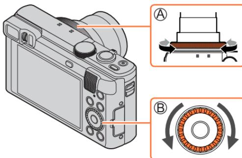
Items that can be set by the control ring/control dial vary depending on recording modes. Following are the pre-assigned settings.
