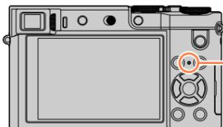
Lit: When the Wi-Fi function is ON or connected by Wi-Fi
