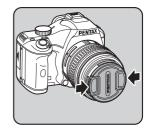
To detach the lens, hold down the lens unlock button (4) and turn the lens counterclockwise.
