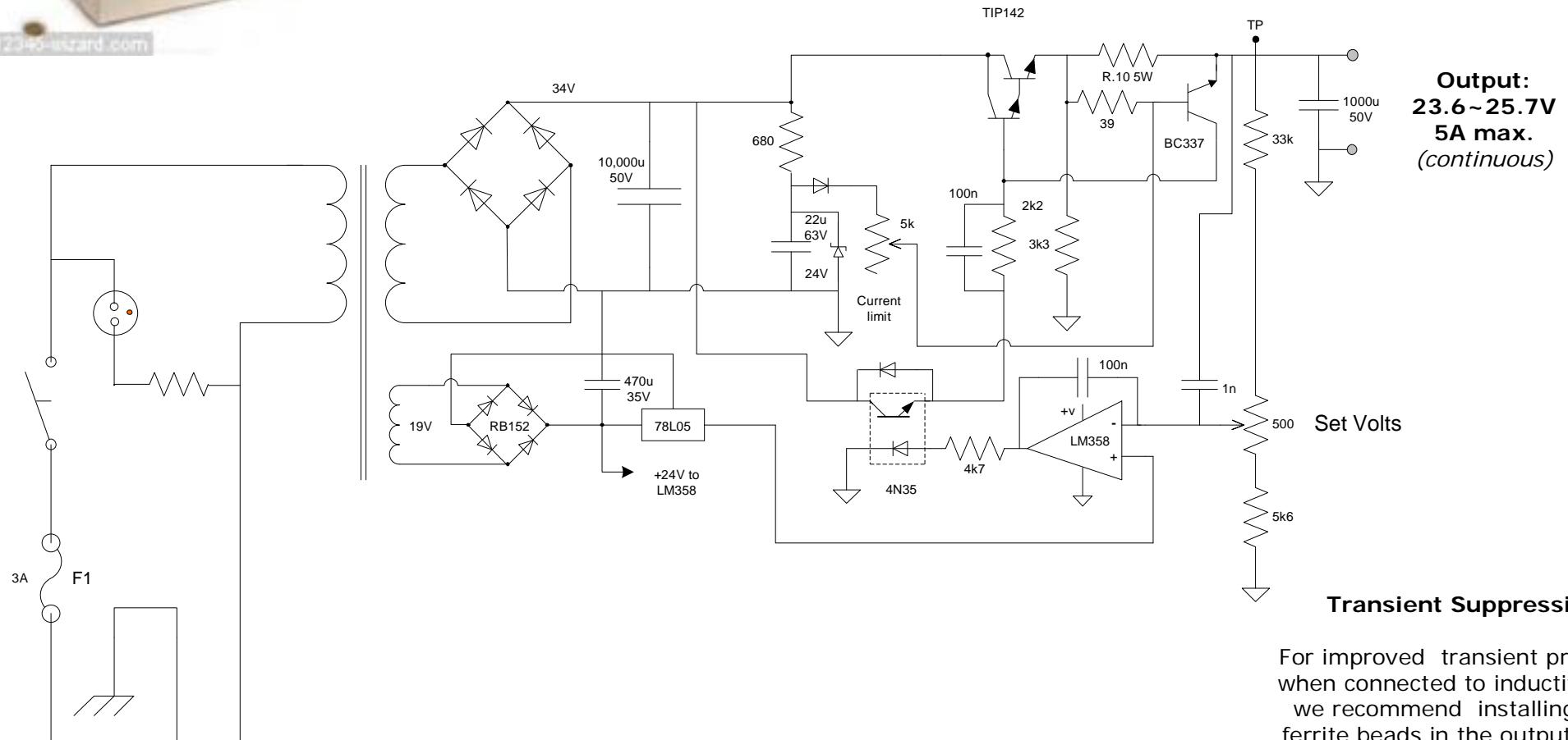
For improved transient protection when connected to inductive loads we recommend installing some ferrite beads in the output circuit.
