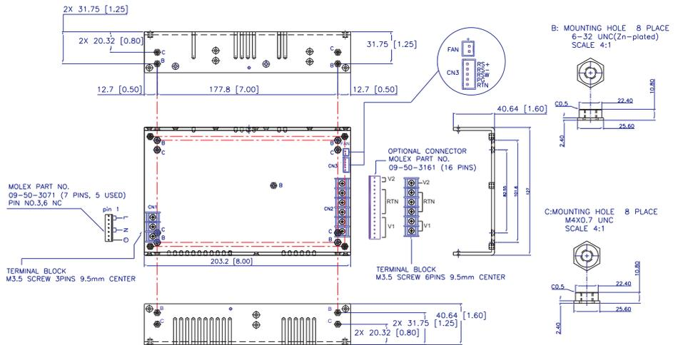
**RL040D2DE Series (Enclosed with built-in fan type): 9 (L) x 5 (W) x 1.6 (H) inches**
