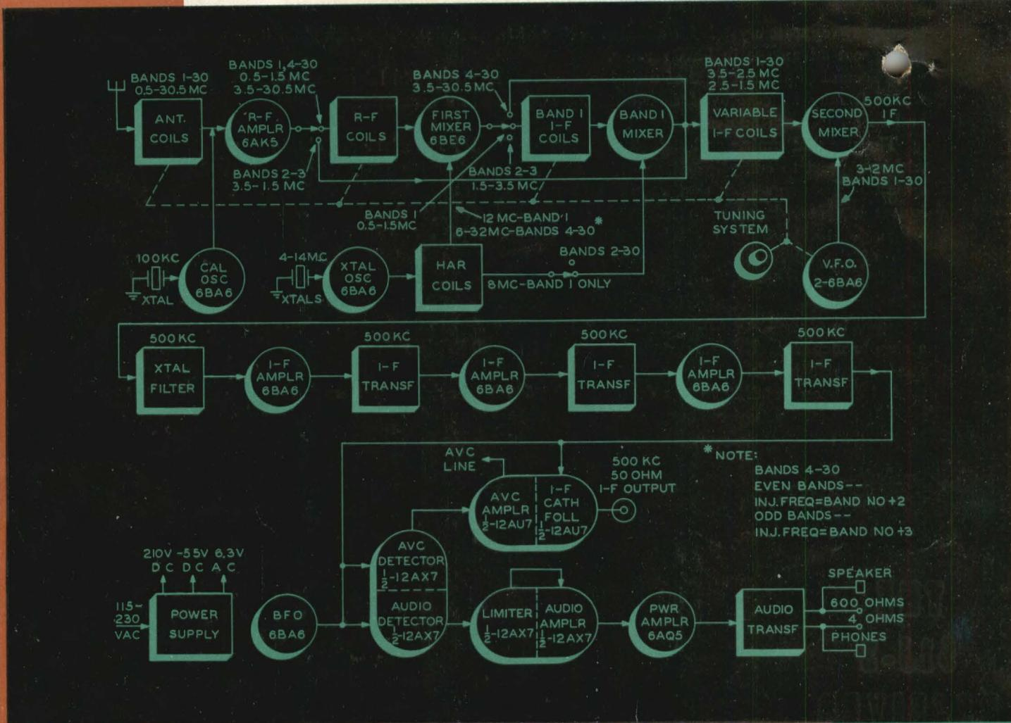
This block diagram shows the frequency system of the 51J receiver. A total of 10 crystals are used to provide stabilization of the first conversion oscillator
