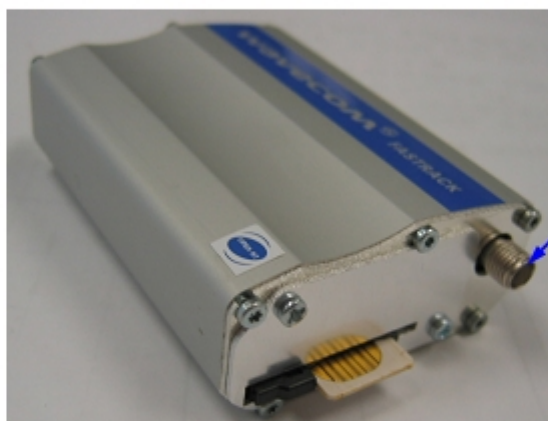
Figure 6: SMA connector for antenna connection
