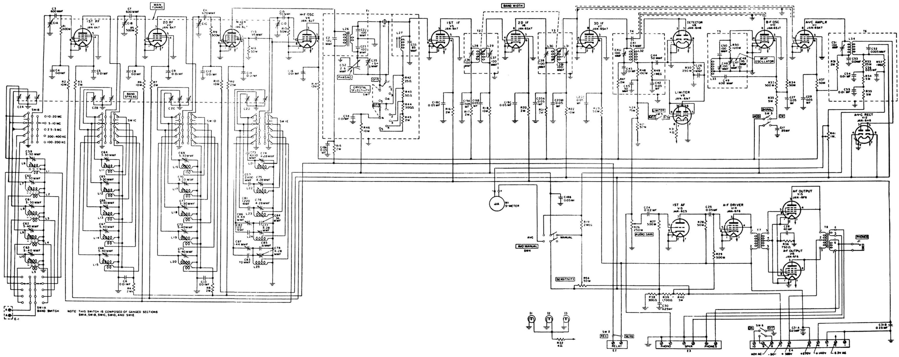
Schematic Diagram, Receiver BC-779-A, B
