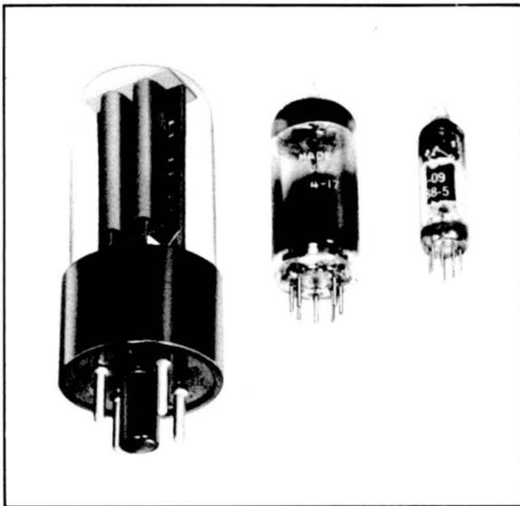
*Subminiature Tube Compared with Standard Tube*
