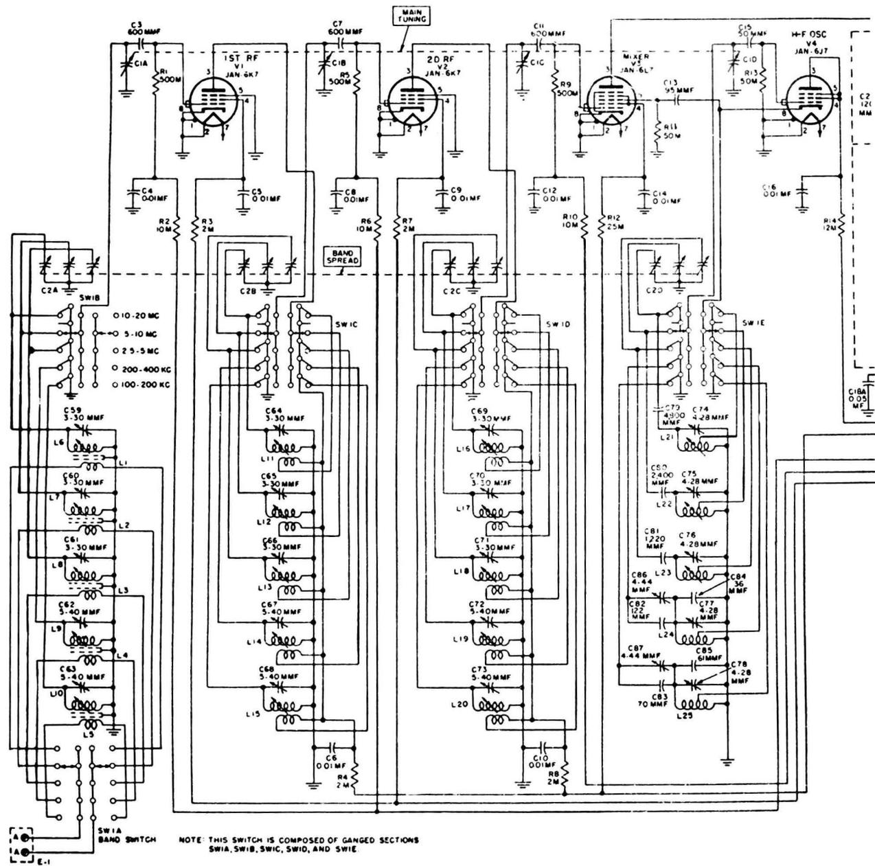
Schematic Diagram, Receiver BC-779-A, B
