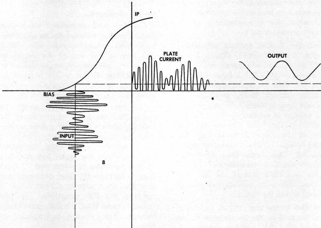
Plate Detector and Response Curve
