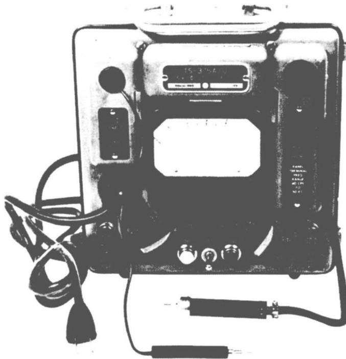
*Vacuum Tube Voltmeter TS-375A/U*
