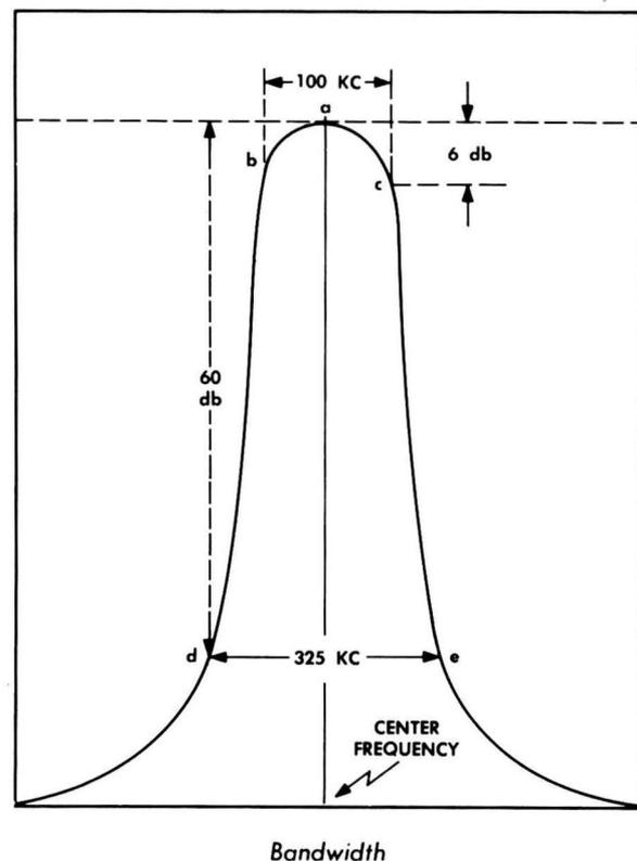
If this bandwidth is greater than 100 kc, the frequency response is too broad. In either case, the alignment should be rechecked. Weak or bad tubes can also account for improper bandwidth.
