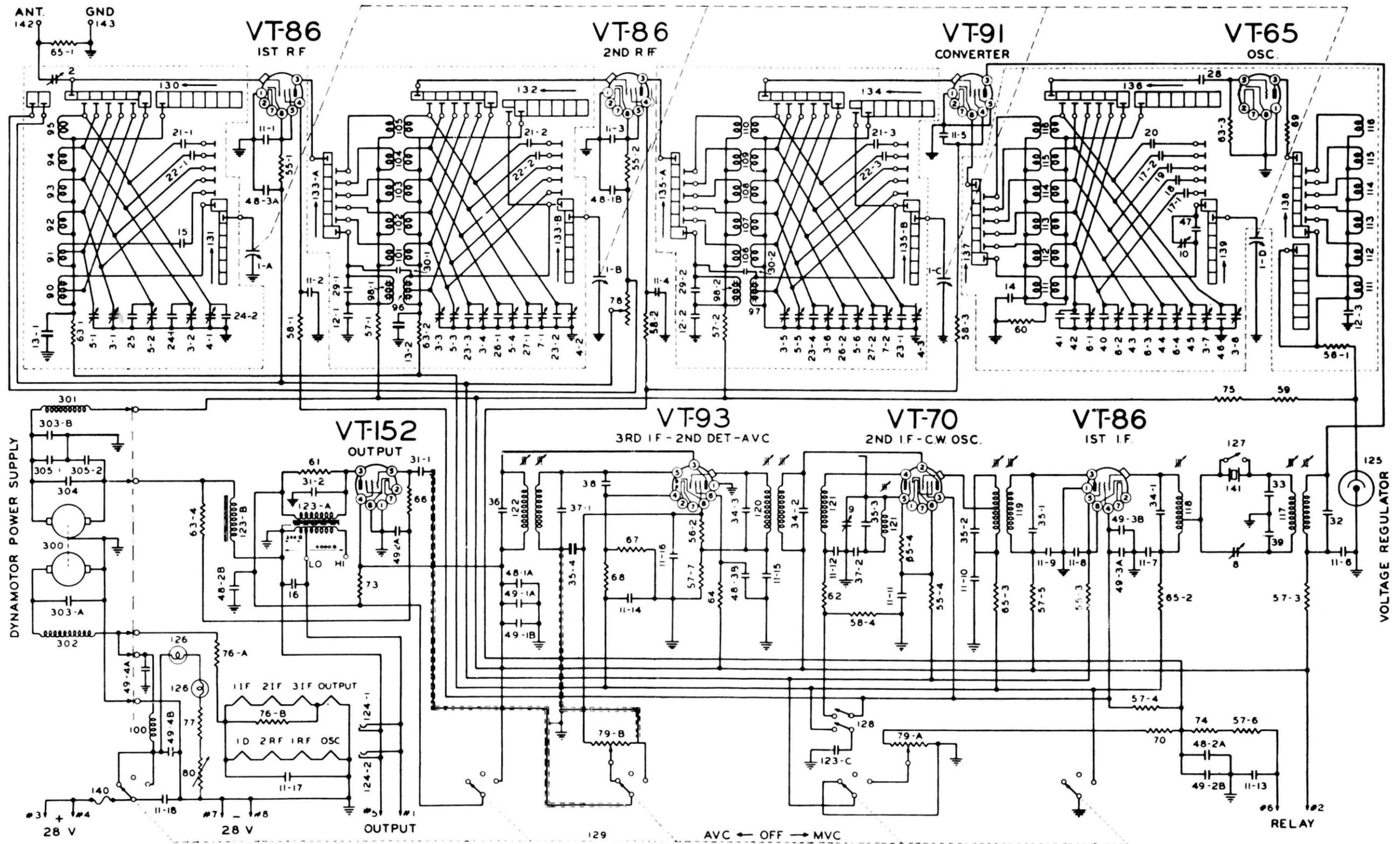
Schematic Diagram, Receiver BC-348 AL
