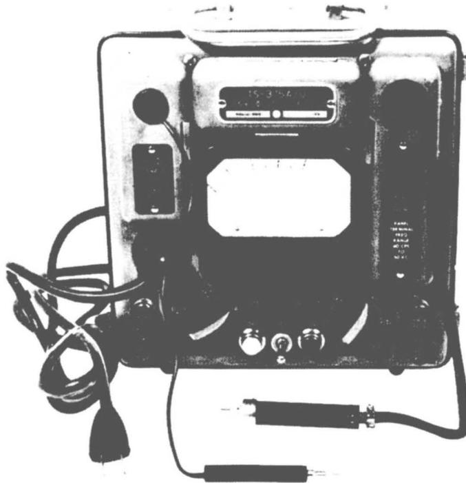
*Vacuum Tube Voltmeter TS-375A/U*
