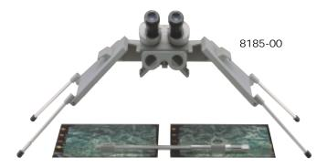
The TRA2 Track Attachment permits work to be carried out over a much wider area and is particularly useful when working with multiple or continuous photographs, since the whole area of the photographs can be examined without interruption. In addition, the Track Attachment permits the instrument to be used to draw contours and to function as a sketchmaster for making maps from photographs by means of parallel translation.
