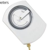
$8025-750 \pm 90^{\circ}$  scale on the left,  $0 \pm 150\%$ scale on right; reads directly to 1/6 of one degree or 1/5 of one percent; skylon case. 8025-90 Similar to 8025-75 except 0  $\pm$  90° scale on the left and scale for direct reading of height of objects on the right; right scale reads directly to  $\pm$  200' at 66 ft.; skylon case.
