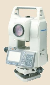
Display unit: Alphanumeric / graphic dot matrix LCD (120x64 dots, 20 characters x 8 lines) on each face, backlight, non-reflective glass, provided. Battery life = 5.5 hrs. per BDC35 battery
