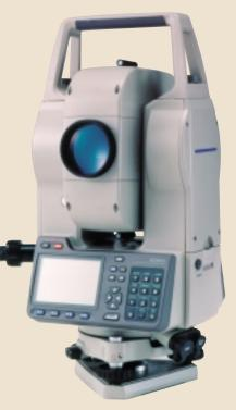
The NET2100 has a large internal memory (448KB) capable of holding a full 3,000 data points. Multiple job files allow a maximum of 24 different jobs. Point numbers can be input alphanumerically. Store 40 feature codes (max. 16 characters each) in memory for easy recall for recording. Measurement and recording are performed simultaneously with a single touch of the "AUTO" key.
