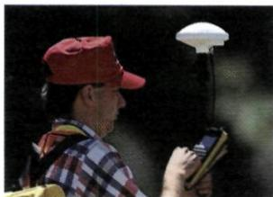
Just slip the six pound receiver into its shoulder pack, attach the new lightweight rangepole/antenna and you're mobile. The new TRK48 keyboard provides remote control of the receiver and lets you enter attributes for every point you survey.
