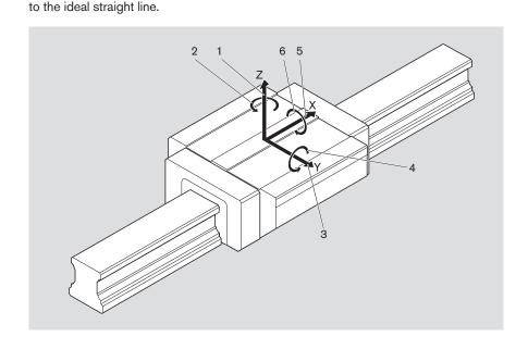
Ideally, the ball runner block should move in a straight line along the guide rail in the direction of the X-axis. In practice, however, deviations occur in all six degrees of freedom. Travel accuracy is the term used to describe the closeness of the movement
