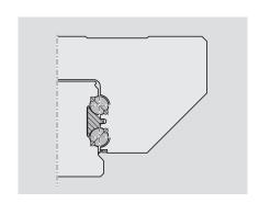
Rexroth's special design with 4 ball circuits ensures that the balls make **contact at two points** regardless of the direction of loading.
