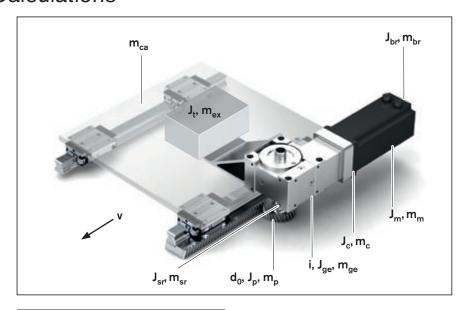
Mass moment of inertia of mechanical system  $\boldsymbol{J}_{\mathrm{ex}}$
