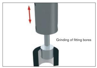
Internal cylindrical grinding
