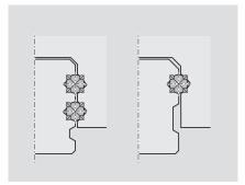
Other ball rail systems with 2 or 4 ball circuits with **4-point contact** have multiple friction: in the Gothic-arch raceway profile, the differential slip at side loading, as well as with comparable preload without load, causes higher friction (depending on the conformity and load, this may be up to approx. 5 times the frictional value).
