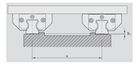
The tolerance for dimension H ("Accuracy classes and their tolerances"  $\mathcal{F}$  26) must be ducted from the permissible vertical offset  $S_1$ .
