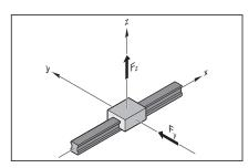
$F_{comb}$  = combined equivalent dynamic load on bearing (N)
