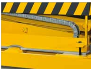
Steel cable carriers on a scissored coil lift Photographs: SKO Steiner GmbH
