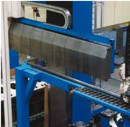
■ Cross-beam cover at a milling machine
