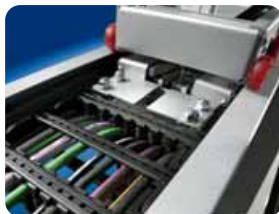
Automatic emergency cutout with decoupling of the cable carrier
