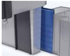
■ Movable chip protection walls (vertical and horizontal)
