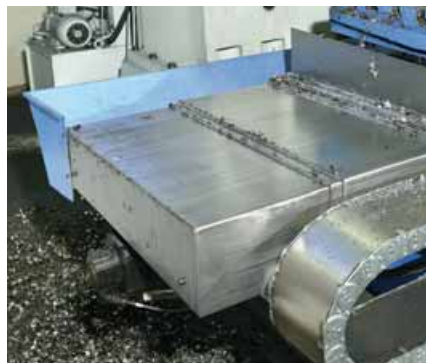
■ Telescopic cover at a milling machine
