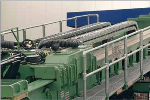
Steel cable carriers on a drilling system
