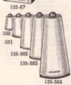
Of the insulators appearing under the headings "Steatite" all but the 500 series and the 135-55 are offered in this finer material for the first time. Their dielectric losses are but a fraction of those for the same parts in porcelain, and they are particularly recommended for high frequency work.
