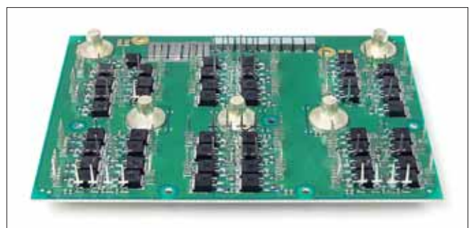
(48) FETs (9) Low profile capacitors (5) Low profile bus bars Total Weight 0.82 lbs (370.6g)
