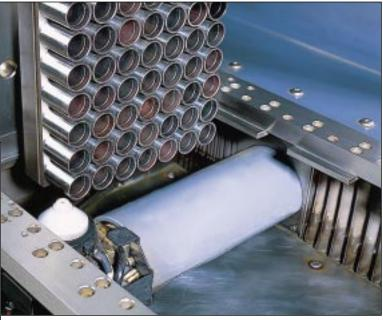
Cutting a pallet of thrust bushings using Electrical Discharge Machining (EDM).
