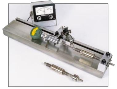
Inspection of bearing for thrust plane error.
