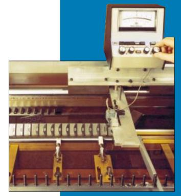
Lead inspection in temperature controlled oil bath.
