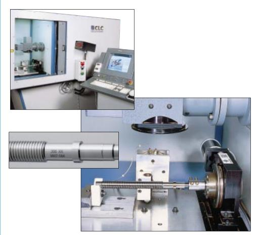
Serial number, lead, and accuracy etched into lead screw and nut with a Laser Marking Machine.
