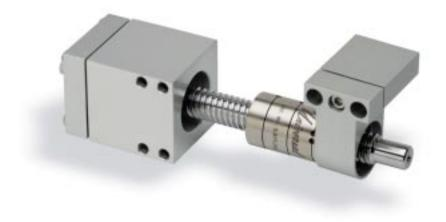
Universal mounting brackets provide proper support and alignment for the thrust bearing and the nut. The lead screw axis and nut clamp are accurately parallel to flat mounting and banking surfaces. The optional motor bracket can be used with the thrust bearing bracket for simple, prealigned motor support.
