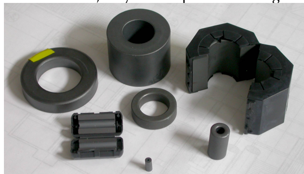
Fig 5 – Ferrites are made in many forms
