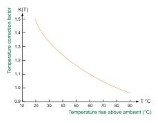
Please note that the thermal performance at different temperature rises, varies from heatsink to heatsink and that the correction factor K is useful as an approximate guide only.
