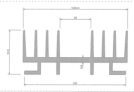
This DOUBLE SIDED Heatsink with internal fixing flanges/feet has been designed to satisfy general purpose applications for MEDIUM DUTY Audio, Industrial or other Semiconductor Medium Power Devices.
