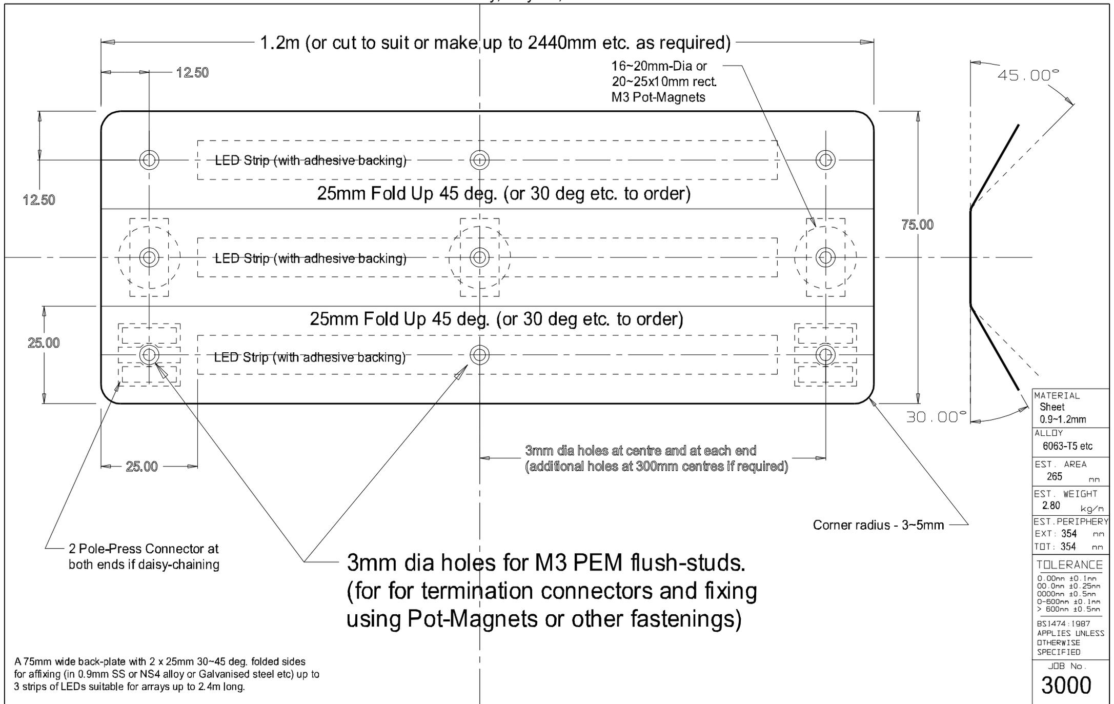
A 75mm wide back-plate with 2 x 25mm 30-45 deg. folded sides for affixing (in 0.9mm SS or NS4 alloy or Galvanised steel etc) up to 3 strips of LEDs suitable for arrays up to 2.4m long.
