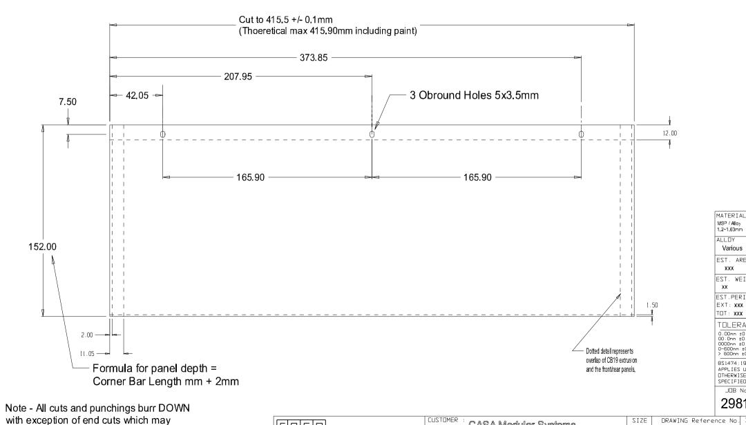
WEIGHT EST.PERIPHER TDT: XXX TOLERANCE 0.00nm ±0.1nm 00.0mm ±0.25mm 0-600mm ±0.1mm > 600mm ±0.5mm BS1474:1987 APPLIES UNLESS DTHERWISE SPECIFIED
