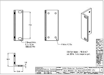
Note - Maximum equipment width is 17" = 431.8mm when using 3mm thick brackets.
