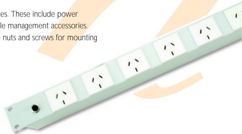
The horizontal units mount in any 19" cabinet. A pair of 23" to 19" adaptor brackets are needed to mount the horizontal units in a 23" cabinet. The 11290007 mounts in any 19" or 23" E or Q cabinet. The 11290008 mounts in any 19" or 23" E or Q cabinet where the cabinet height is 1800mm or 2100mm. These units come with a 2m cordset and are equipped with 10A sockets and a 10A B Curve MCB.
